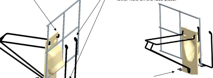
**Step 3: Fasten to Fence:** Tighten wing nut onto stud at base of u-shaped wire support bracket.
